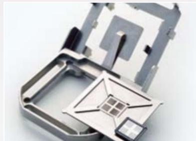
QFN prebumping mask / frame and solder paste printer.
