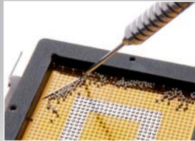
Easy distribution of solder spheres (solder balls) on a universal mask. Excess spheres are simply poured back into container.
